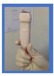
Cover transducer (including footprint) with tight plastic wrap (transducer cover or condom) and gel
